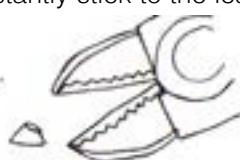
The excess leads are useless, cut them off with a flash cutter. Here you go. Finish all leads of resistors now.
