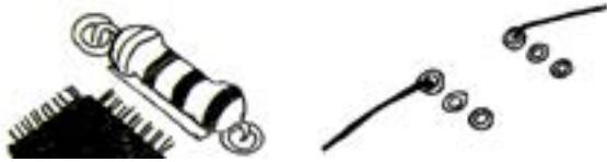
Flip over the base board and bend away its two leads. This way we can fix the component onto the board so it won't move when the board is flipped. Now follow the table to insert all resistors.
