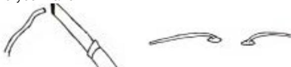
Now let's start soldering our first pad. Place the solder against the pad you want to solder. Move the tip of the soldering iron to the pad and melt some solder. The melted solder should instantly stick to the lead and form a volcano shape.
